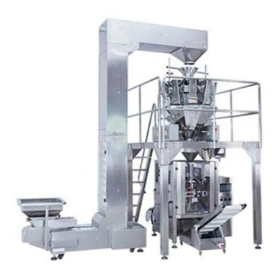
This production line is mainly composed of bag fully automatic packaging machine combined with electronic scales, bucket elevator, work platform supporting and become, is suitable for candy, nuts, raisins, peanuts, melon seeds, nuts, potato chips, chocolate, cookies and other big particles and sachet big bags, such as radix isatidis granule packing a big pack of automatic measurement.
