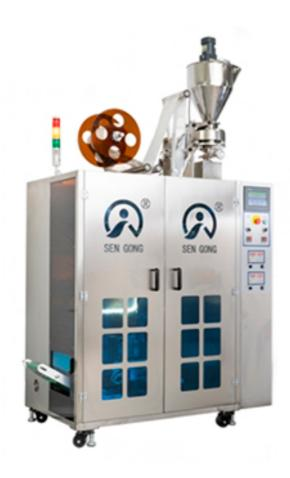
C19H Guatemala Drip Coffee Packaging Machine With Outer Envelope is suitable for inner and outer bag packing granule coffee, coffee powder 5 to 15 gram coffee inner and outer bag packaging.
