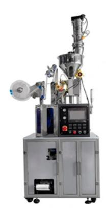
The machine adopts automatic following, automatic tracking, automatic positioning, and other systems; no excessive intervention in parameter setting or adjustment is required during working; With One-click power-on, one person can operate multiple units; This type of drip coffee packaging machine is equipped with a fully automatic loading system and uses a special surface treatment process for slide doser unloading to ensure gram weight accuracy.
