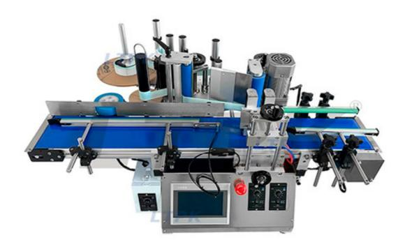
This automatic bottle labeling machine is with a conveyor and it has similar functions like the full automatic labeling machine. This round bottle labeling machine can be used for double side labeling. The desktop type labeling machine can save working space. It is widely used to label round bottles like wine bottles, toner bottles, food cans etc.
