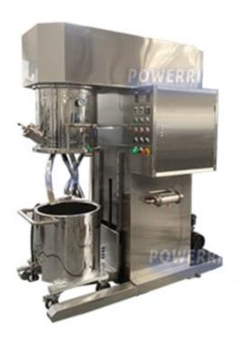
The double planetary mixer is a specialized industrial mixing equipment designed for efficient blending, dispersing, and mixing of various materials. It consists of two blades or mixing agitators that rotate on their own axes while simultaneously orbiting a central axis. This unique movement pattern enables thorough and uniform mixing throughout the entire batch.
