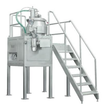
GM Series high shear mixer granulator is used in pharmaceutical solid dosage area for mixing and granulation application. It's the major processing equipment in solid dosage production line. The equipment is PLC automation controlled and well satisfies the current GMP and Pharmacy Code regulation.
