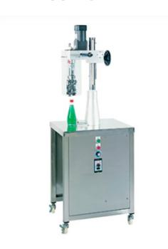
The container cap sealing equipment is semi-automatic capper. It is suitable for object container with aluminum caps.
