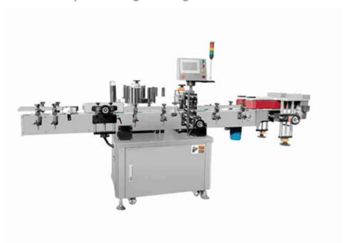
Bottle feeding  $\rightarrow$  cylinder bottle clamping  $\rightarrow$  batch number printing  $\rightarrow$  spotting and positioning labeling  $\rightarrow$  testing and rejecting  $\rightarrow$  finished product. This equipment is suitable for fixing and positioning labeling of large round bottles made of glass, plastic, metal, etc. (such as large infusion bottles, penicillin bottles, eye drops, syrup bottles, wine bottles, paint buckets, etc.).
