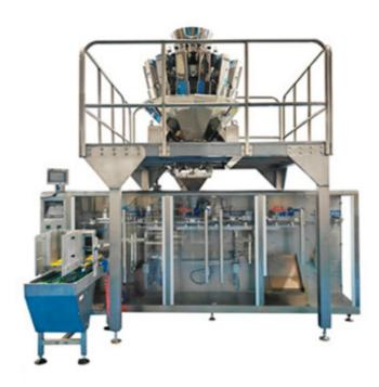
The machine is an automatic packing machine for premade bags. It can meet the requirement which needs different specifications, big or small volume but small capacity. It can not only pack 3-side or 4-side sealed bags but even also bags with hanging holes, standing pouches shaped bags doypack bags with corner spouts, etc. It is applicable to powder, granules, liquid, paste blocks, etc by using different measuring devices. It is convenient to switch the packing type.
