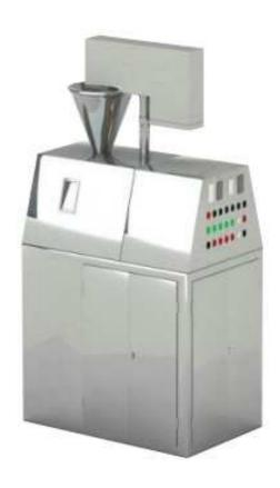
As a new equipment, GK Dry Granulator utilizes the crystallized water in the material to pelletize the powder into granulate, this machine features novel and reasonable structure, stable and reliable performance, easy maintenance and cleaning. Granulates made by the machine can be pressed into tablets or capsules, and it's mainly used for granulation in pharmaceutical, chemical, foodstuff and other trades, esp. for granulation of materials not suitable for wet method.
