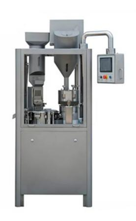
NJP-800 automatic capsule filling machine operates intermittently and fills capsules with a metering plate of holes. The machine is bettered and designed, considering features of Chinese medicine and requirements of GMP. As a result, the machine is characterized by compact structure, small size, low noise, accurate filling, perfect functions and stable operation. Meanwhile, it can feed, separate, fill and lock capsules, clean wastes, discharge end products and clean molds synchronously.
