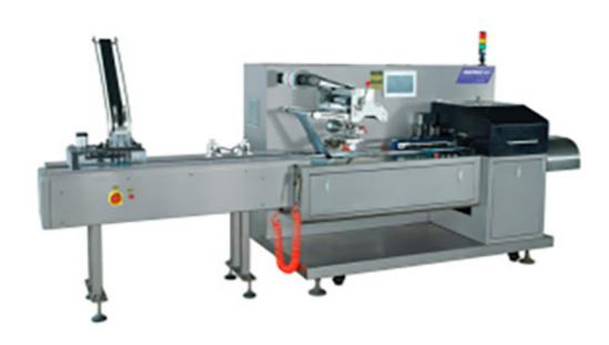
GZP-180 New type High Speed Flow Packing Machine, adopt full servo motor drivers, Reciprocating type sealing design, use High sensitive photoelectric eye color tracking system and other advanced institutions, Garantee the quality and safety of medicine packaging, advance the packaging product efficiency. It is mainly applicable to the packaging of medicine plate, biscuit, betel nut, snow cake, instant noodles, candy, pastry, bread, pallet container, transparent soap, etc.
