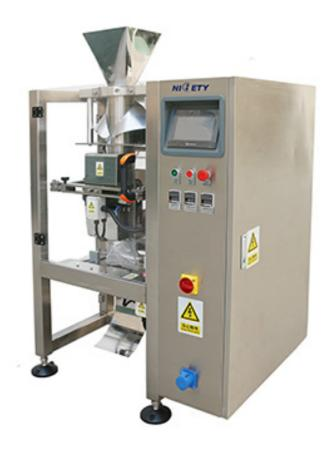
The film passes through the molding unit and complete bottom seal and vertical seal, after filling the materials to the pouch by the buffer hopper, complete the top seal and cut to get the final products.
