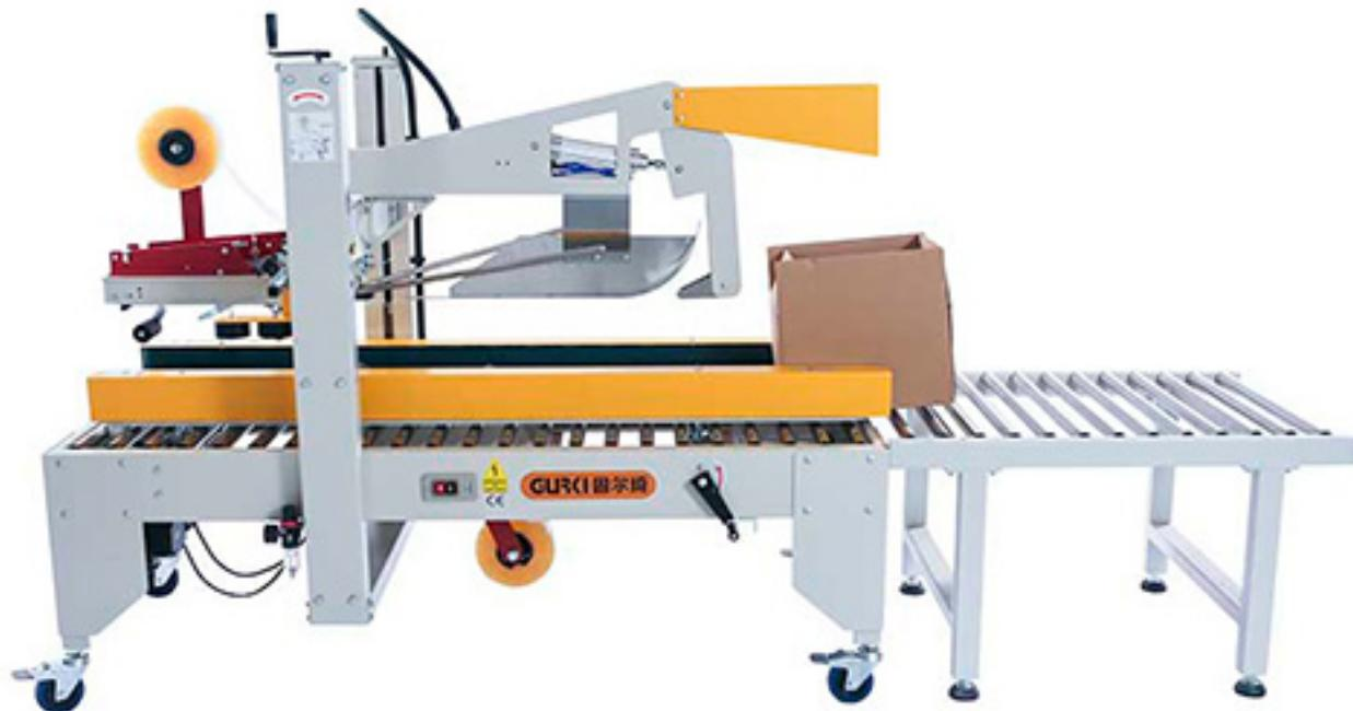
Semi-auto flaps folding carton sealer GPC-50D automatically attaches the tape to the top and bottom, no need for manual work. It uses adhesive tape to seal the carton, not only the sealing effect is beautiful, and the sealing is firm. The use of the automatic packaging line will better reflect the value of this machine. This type of sealing machine is widely used in food, medicine, beverage, tobacco, daily chemical, automotive, cable, electronics and other industries at home and abroad.
