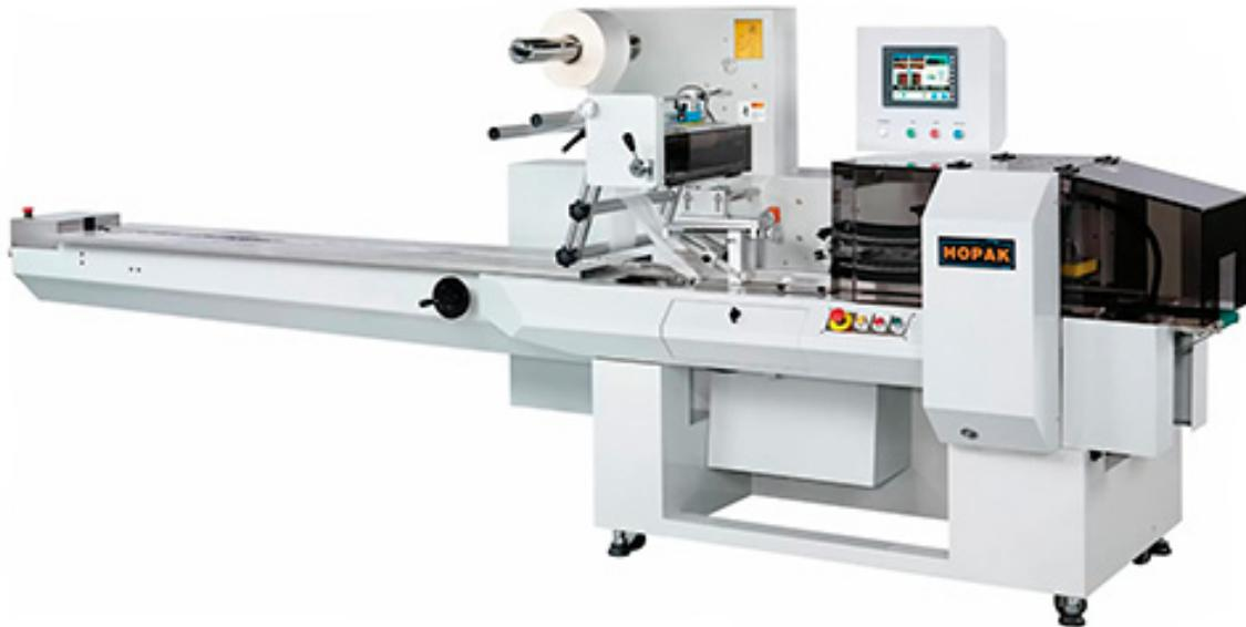
D-cam Horizontal Flow Wrapper designed for bigger and higher product, options for gusseted device to make packaging appearance more attractive.
