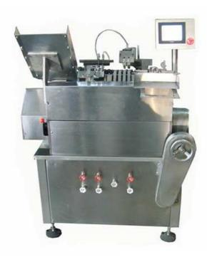
The machine is a new generation of the ampoule drawing, filling and sealing combined equipment for injections. It adopts the rectangular feeding instead of the traditional ampoule feeding methods. In such case, the feeding is steady with no easy broken ampoule. A modern clutch is mouthed under the ampoule feed hopper.
