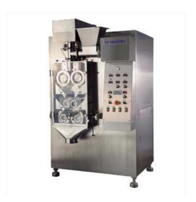
The roller compactor is designed for precide adjustment of three variables to allow for different kind of material. The three adjustable variables are Screw Speed, Roller Speed, and Roller Pressure; the calculation fo bulk dansity is related to adjusting of the roller gap, the screw speed and the roller speed. The capacity differs depending on the bulk density of the materials according to the following equation.
