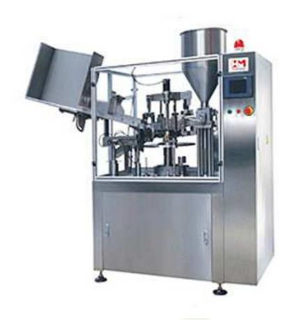
Usage: suitable for filling and sealing Alu. tube or plastic tube with cream or ointment.
