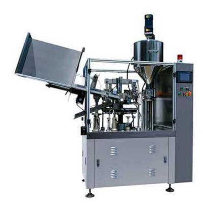
VZ-60Z Metal Tube Filling and Sealing Machine can be used in the industries of pharmaceutics, foodstuffs, cosmetics, daily chemicals for smoothly and accurately filling all kinds of pasty and viscous fluid and the materials alike, into soft metal tubes and then carrying out tube end folding, sealing and lot number printing.
