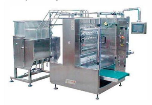
As shown in the picture, the packing machine is used for packing catsup and other thick paste materials such as peanut oil, salad oil, tomato paste, cough syrup, shampoo, cream oil, vaseline and so on, providing measuring and automatic packing into sachets. It is used in the medicine, food, daily chemical and other industries.
