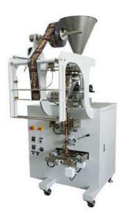
This model is facilitated with various sides sealing, which guarantees complete safety. This is designed for fast and easy changeover and thus packaging is done fatly. Electronic web edge control with excellent sensitivity and high precision is installed in this model and closely monitors and controls the wind and unwinding of the bags keeping an edge in the correct position.
