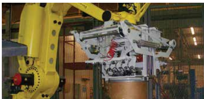
One end effector including ring gripping device for drums and finger gripper for bags
