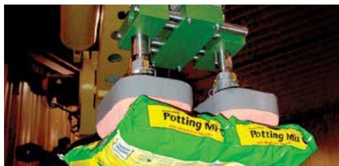
Vacuum gripper for bales, bags or boxes
