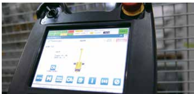
Color teach pendant used as main interface on standard cell
