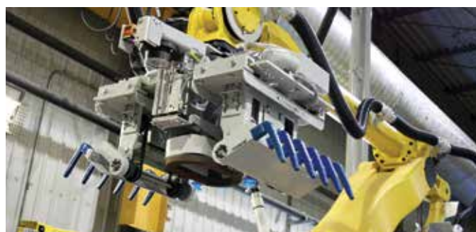
Dual function gripper: finger for palletizing and vacuum for depalletizing
