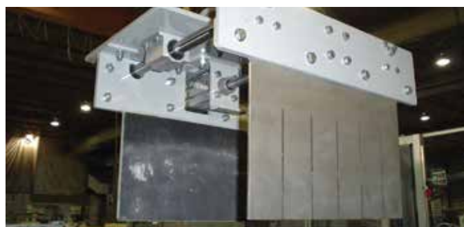
Bundle gripper with bundle height measuring system to compensate product density variations
