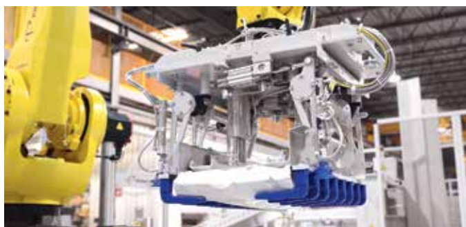
Finger gripper equipped with optional automatic bag width adjustment system
