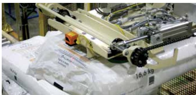
Vacuum gripper with pallet handling option
