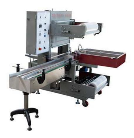
SA-117 & SA-117-1 sleeve sealing machine (not including shrink tunnel) is suitable for products in one tray pack, single carton or some simple collections of large products. Available with transparent PE shrink film (each Top and Bottom film cradle) OR printed PE film (only Top film cradle) Its speed could up to 16PPM or 12 PPM depends on the product dimensions.
