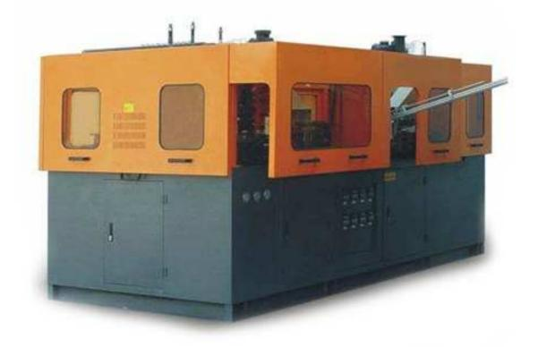
The Main Application of Semi-automatic Blow Molding Machine is to produce wide range shapes of PET/PC/PE bottles. It is able to produce from 100ml -6000ml bottles, which is widely used producing all kinds of bottles, including mineral pure water bottles, mineral water bottle water, carbonate soft drink bottles, juice bottles, medical bottles, cosmetic and oil bottles etc.
