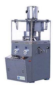
This tablet press is a single press type, continuous automatic tablet press for pressing granular raw materials into tablets. The rotary tablet press is mainly used in pharmaceutical, chemical, food, electronic, plastic and metallurgical industries.
