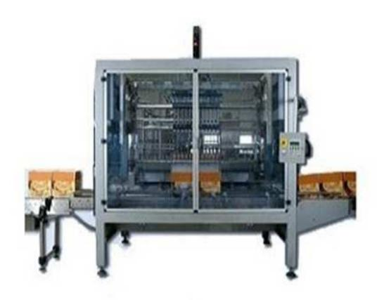
Electric packer machine is of intelligence automation equipment, it adopts P.L.C control, and touchable screen control, with ultrahigh depart device to pack all kinds of container, plastic bottle, regular and irregular bottles, and other packed boxes with extra boards. The bottle pins seize the bottle and relax in the carton. It is widely used within production line for it has reduced labor tension and improved the packing efficiency.
