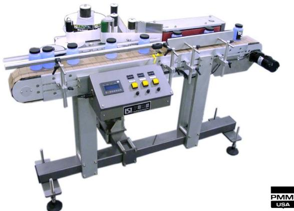
The Series 1500 is LSI's line of labelers specifically designed for wrap around labeling of products such as bottles, vials, or cans. The **Series 1500** is designed to work with any of LSI's standard labeling heads such as the Series 40 Apply Only Labeling Head and Series 20 Print & Apply Labeling Head. The Series 1500 includes such features as:
