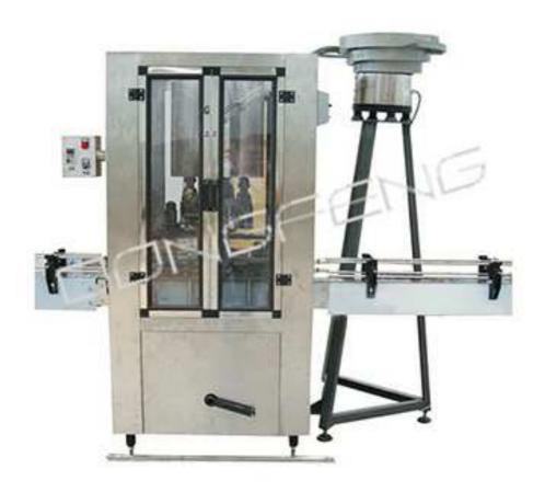
This is our newly developed capping machine, integrates bottle inlet, cap sort, cap feed, capping, bottle outlet together. Well suitable for diversified caps, also very friendly applicable for anti-theft caps. Caps are grasped and positioned well, harmless to caps during the machine running. Fast speed of machine and high qualified rate of capping, it bears step less adjusting, can reach the international advanced level of similar products.
