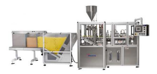
The ProTrac system with speeds to 220 tubes per minute features a race track design, dual filling and closing stations as well as multiple post filling options.
