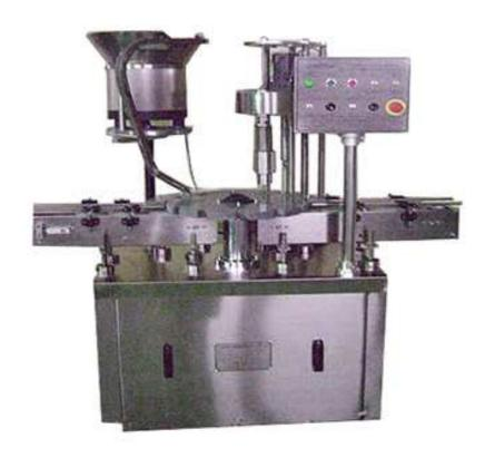
This machine designing based on many years experience for producing capping machine, especially suitable for the threaded cap, unique structural design, three cutters for cap sealing, stable performance, can replace similar imported machines, preferred machine for capping high-level products.
