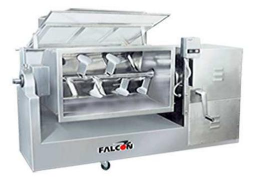
Salient Features: All contact parts are made of SS 304 (SS 316 optional) Thrust bearings are provided to carry rigid and thrust load. Easy for cleaning and operating. Interlocked acrylic dust cover for inspecting the mixing process. The tilting device provided for easy unloading of the material.
