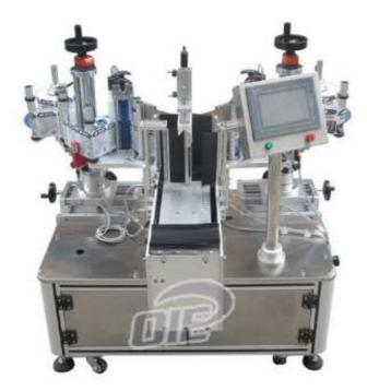
OL-909 is a fully automatic linear labeling machine well designed for round bottles, oval bottles and square bottles single and double sided labeling, such as shampoo oval bottles, lub oil bottles and hand washing bottles.
