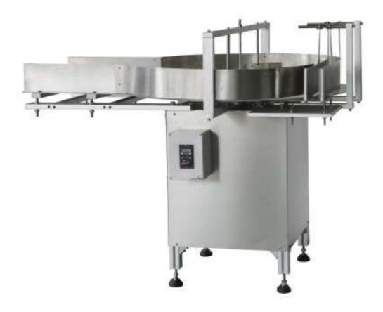
Bottle feed-in turntable is used in a wide variety of bottle packaging or filling production lines. In general, rotary table is connected with the beginning of production line to feed round container into the packing line. The bottle moves along the table edge which could greatly reduce the possibility of bottle jamming.
