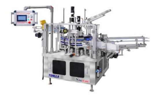
The new series cartoning machine built with "BALCONY" design, allowing the mechanical working parts separated from the packaging area. It respects the present accident prevention maintenance and hygienic laws. The machine works with intermittent motion and with electric synchronisms controls, PLC and touch display control system functions recall-able; it is possible memorizing 100 menus with relative data for 100 different productions.
