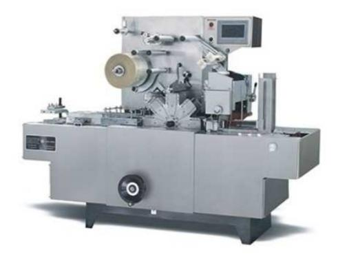
An overwrapper machine takes a length of heat sealable film from a roll and folds it around a product. This product can be a single item or a bundle. The folded film is closed by means of heated sealing devices.
