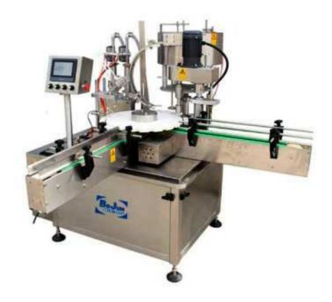
The equipment is automatic filling and capping machine, which makes the high-viscosity filling and ordinary pressure filling into one. Under the high-viscosity mode, the machine adopts the cylinder to control filling head so that it can ensure the stability and precision; under the ordinary pressure filling mode, the filling part adopts fixed passageway parameters, and the machine realizes the different filling dose by controlling the filling time.
