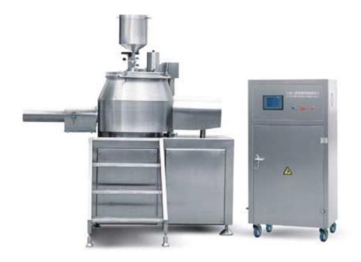
With PLC Full-computer Automatic Control produced by German Siemens Co., this system has friendly man-machine interface, screen cue operation and graphic parameters. Data can be input by simple touch keyboard.
