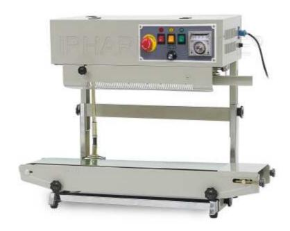
FR series continuous film sealing machines finish continuous carrying, sealing and printing in one operation. Suitable for small-bag packaging, this continuous band sealer uses an electronic constant temperature control system and a stepless speed adjusting transmission mechanism.
