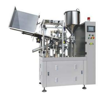
This Tube Filling And Sealing Machine is made of high-quality stainless steel 316L, which is suitable for cosmetics, chemical, food, pharmaceutical and other industries.
