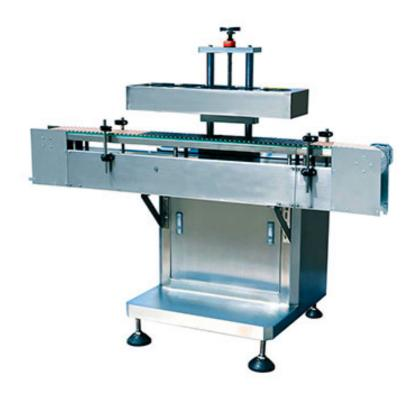
The bottles with aluminium foil pass under the inductive head, the aluminium foil heats after receiving the energy produced by the inductive head. The heated aluminium foil melt the plastic film attached to the aluminium foil and glue to the bottle mouth so it can achieve the sealing effect.
