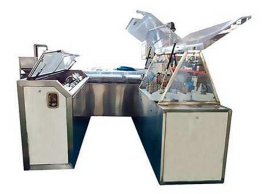
This is a machine that has been developed for the production of suppositories in PVC, PVC+PE. Its working is completely automatic, pneumatically based, controlled by a programmable logic.
