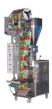
FFS Machine is an assembly-line product packaging system. These machines make plastic bags from a flat roll of plastic film and simultaneously fill the bags with product and seal the filled bags. There are two types of FFS machines namely vertical form fill seal (VFFS) and horizontal form fill seal (HFFS) machines. Our machines have user-friendly controls made with modern technology equipment's such as microprocessor/PLC etc.
