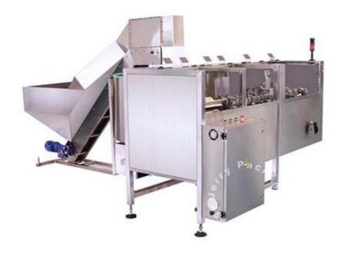
JLP-200H Automatic Bottle Unscrambler is making up of bottle elevator, round plate, bottle rejector, bottle-arranging and the electrical cabinet. Put disordered bottles to the bottle elevator, through round plate, conveying belts, bottle arranging parts, and then bottles can stand on the belts. This machine is characterized by the compact structure, simple operation principle, mature technique and stable movement.
