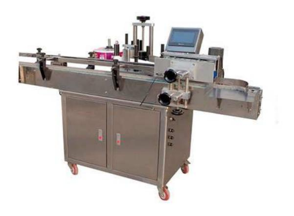
Vertical round bottle labelling machine adopts advanced rolling on label, using computer control, synchronous tracking, label is controlled by the stepper motor or servo motor control, automatically detect the bottle and label size to ensure accurate labeling, automatic synchronization. The machine is controlled by microcomputer, touch type large LCD panel, display and store ten sets memory devices.
