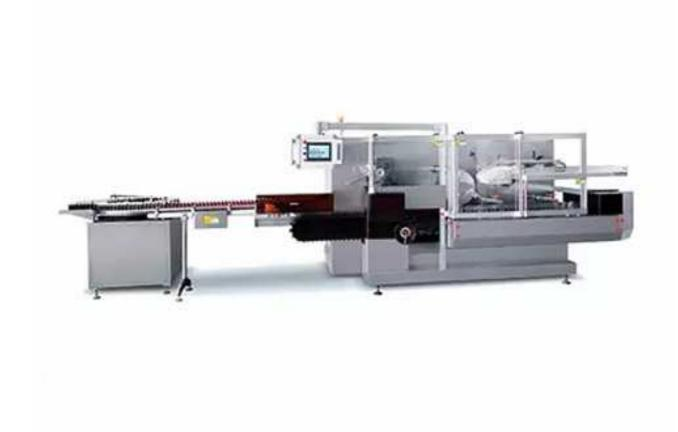
This machine is used to take Alu/PVC medical plate or plastic bottle (vitreous bottle) to filling in paper box automatically. It can perform automatically the whole process of folding and conveying of leaflet, paper box forming, batch number printing and box sealing. The machine can also be linked to work with Alu/PVC packing machine, bottle filling machine and transparent film three dimensional packing machine.
