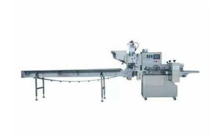
Suitable for packaging of multi-pack of individually wrapped products, such as snow cakes, egg pies, French bread and biscuit, etc. This machine has a wide usage and can change products quickly by simple adjustment, etc.
