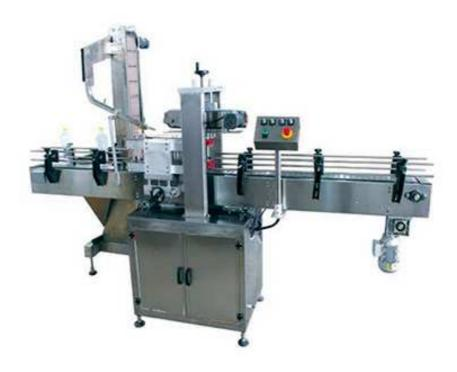
Automatic snap capper machines apply push-on caps, press-on caps, and snap-on caps onto bottles and containers at speeds of up to 150 caps per minute. In addition to snap-on caps, Automatic snap capping machines apply lids, plastic pull up spout caps, over-caps, sifters, dropper inserts, dropper tip plugs, orifice reducers, as well as balls and fitments onto roll-on containers.
