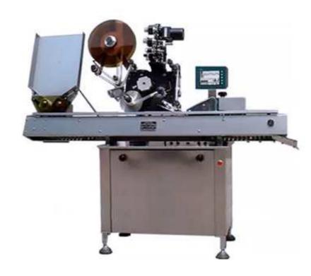
DWTB-C is economical, self contained, easy to operate, equipped with auto teach programming touch screen. Built in microchip storing different job setting makes fast and easy changeover. This automatic labeling system is ideal for slim cylindrical container with diameter from 10mm 25mm such as ampoule.
