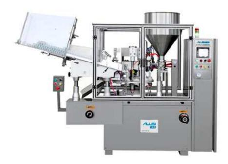
Automatic Tube Filling Machine can perform the filling for ointment, cream jellies or viscosity material, sealing or tail folding, batch number embossing (include manufacture date) automatically. It's ideal equipment for aluminum tube filling and sealing for cosmetic, pharmacy, foodstuff and bond industries.
