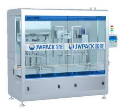
CCG5000-3-1 automatic filling cover is a combined packing machine integrating filling and rotary cover. Suitable for the filling of water agent and high viscosity materials. The whole machine has the characteristics of compact structure, small land area, easy cleaning, easy operation, convenient and fast replacement of quality rules, which can save to the greatest extent human.
